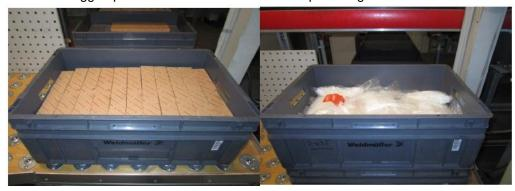
The euro norm container is to be protected from damage and deformation. In some cases, top covers or edge protection should be used.
