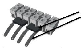
Assembly of the external cross connections QB 2 MK6:
