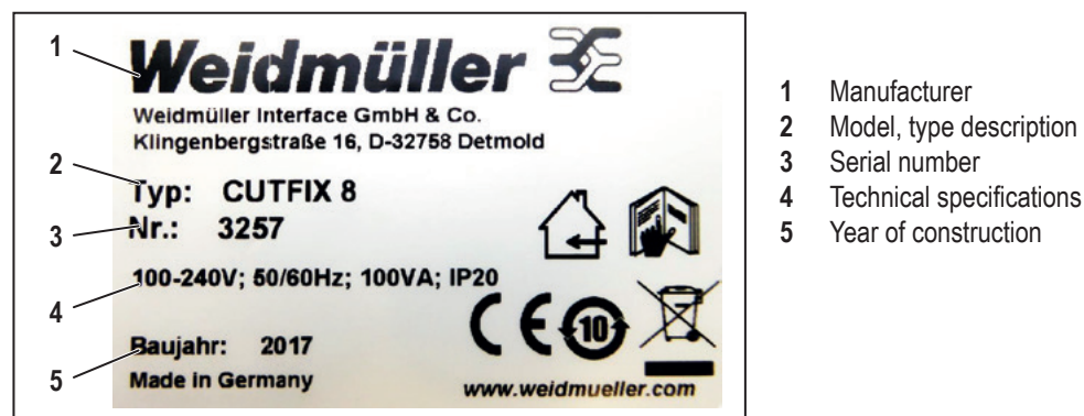
Figure 3.3 Type plate on the rear side of the machine
