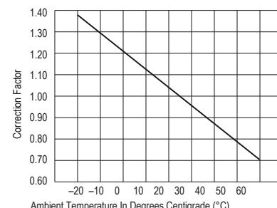
**To use this chart:** Read up from the ambient temperature to the curve, and across to find a correction factor. Multiply the breaker rating by the correction factor to determine the compensated rating. Calculate the overloads in terms of the compensated rating to use the published trip curve.
