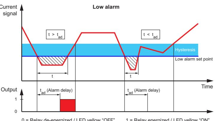
0 = Relay de-energized / LED yellow “OFF”      1 = Relay energized / LED yellow “ON”
