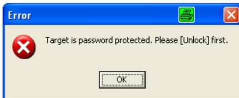
In this case, proceed as follows to "Unlock" the IE-CS(T)-2TX-xRS232/485.
