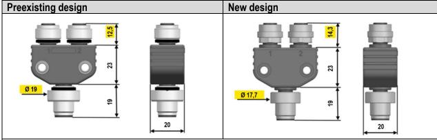
**Note**: the two pins for ensuring the distance during assembly are not shown, **but remain in the new** design with the same dimensions!
