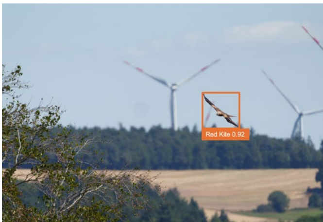
Visualisation of bird detection by AVES Wind anti-collision system with species recognition AI with indication of probability
