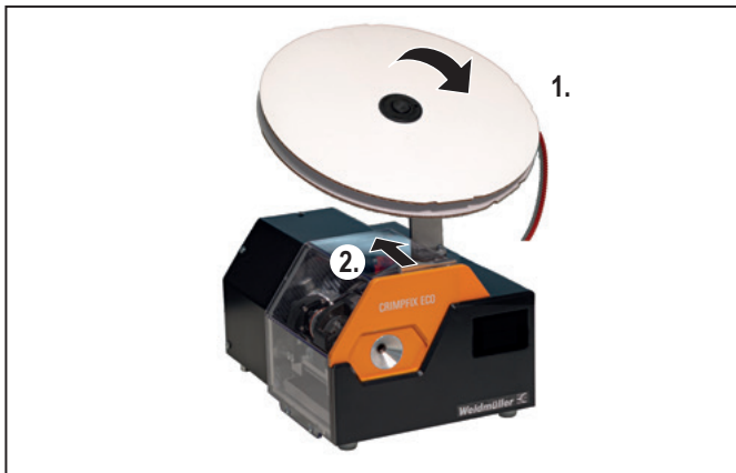
Figure 6.1 Place the wire-end ferrule reel
