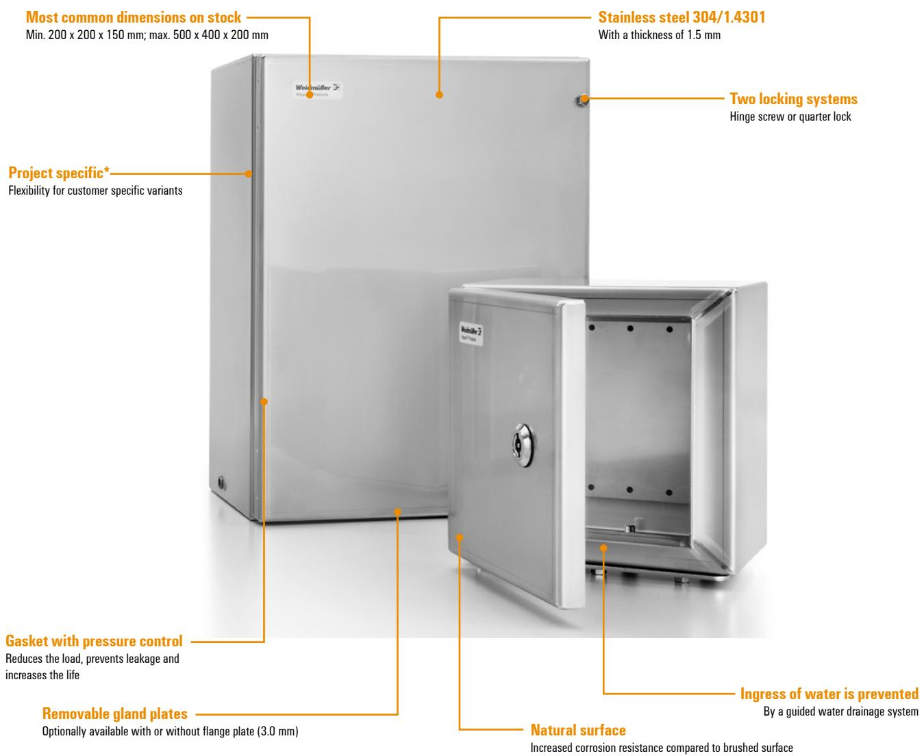
\*Adjustments possible: Materials, surface finishes, material thicknesses, paintings, dimensions, attachments, cut-outs, assemblies
