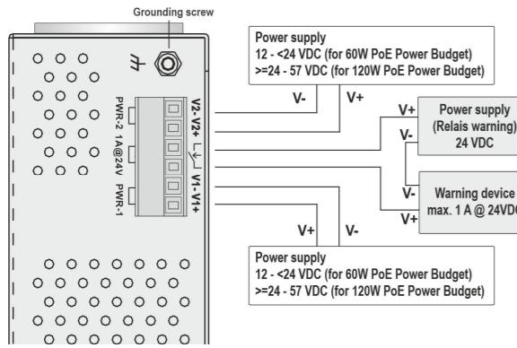
**Behavior of fault alarm relay (can be triggered by configurable events power failure or port link down):**
