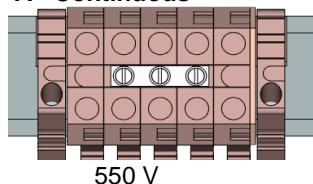
**C - Adjacent – separated by an end plate**
