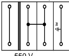
**F2 - Next to a protective conductor terminal (earth) with a partition plate TW...**
