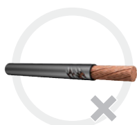
Damaged conductor insulation
