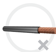
Excessively twisted individual wires
