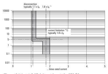
\*1) current limitation typically 1.8 x I $_{\Pi}$  times rated current at I $_{\Pi}$  = 1.0 A...6 A current limitation typically 1.5 x I $_{\Pi}$  times rated current at I $_{\Pi}$  = 10.0 A
