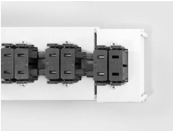
Figure 6: Tolerance compensation is provided by the multi-leg contact spring for device offsetting during installation.
