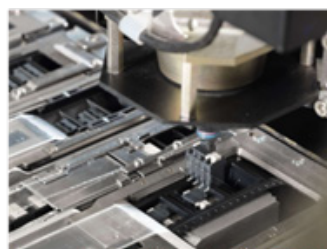
Removal of the component by means of vacuum pipette from the belt ("picking")
