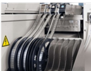
Component feed with tape-on-reel
