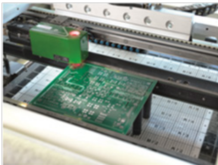
The PCB is transported to the paste pressure station and measured
