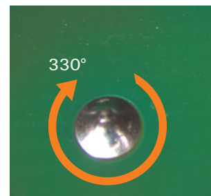
Secondary side: Circumferential wetting and solder wetting
