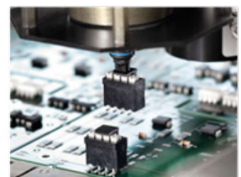
Place the component on the PCB
