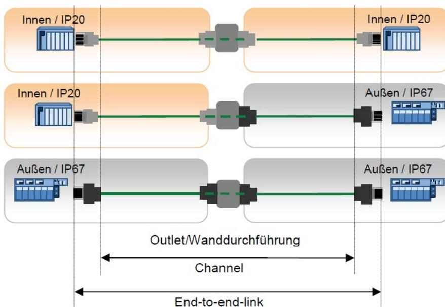
Image 3: Example variants for the End-to-End link in accordance with the PROFINET guidelines.
