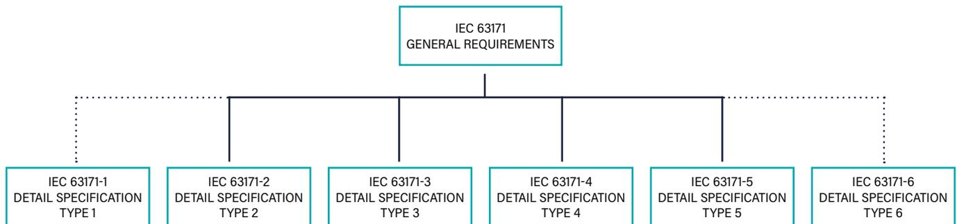
Image 1 outlines the structure of the IEC 63171 series of standards and the normative references to IEC 63171-1 and IEC 63171-6
