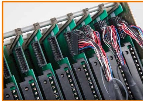
Connect cable with connector to adaptor card
