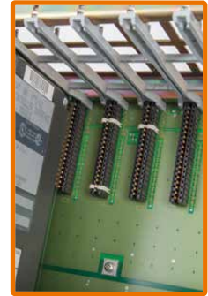
Remove all key codes from the backplane connectors.
