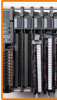
Remove existing Field Wiring adaptors
