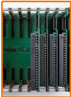
Replace controller card with Weidmuller adaptor card
