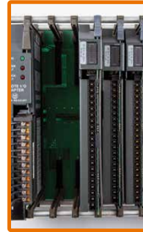
Remove existing controller cards
