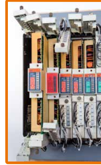
Remove existing controller cards
